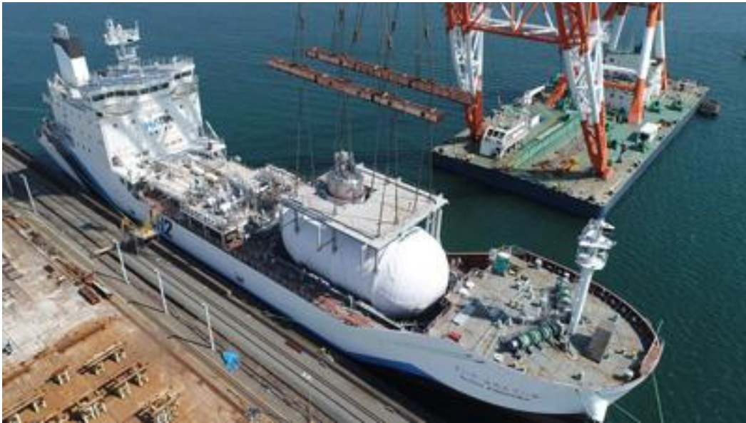
Figure 14 — World's first liquefied hydrogen carrier launched in Japan. This ship of 120m will carry 90t of hydrogen.
